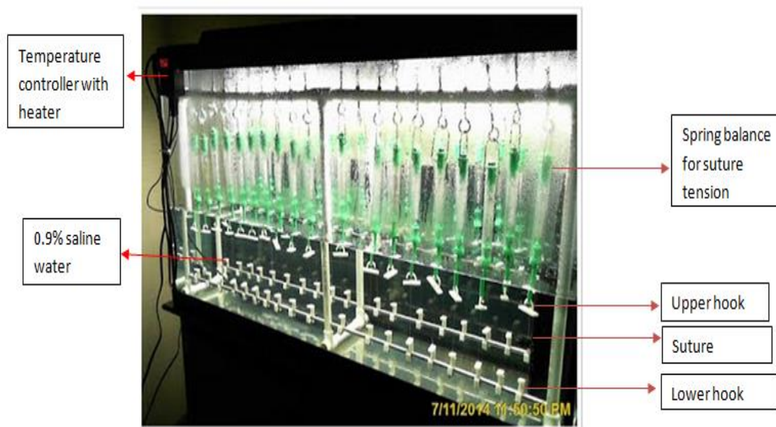
Figure 23: Experimental setup for tensile strength analysis of absorbable suture
