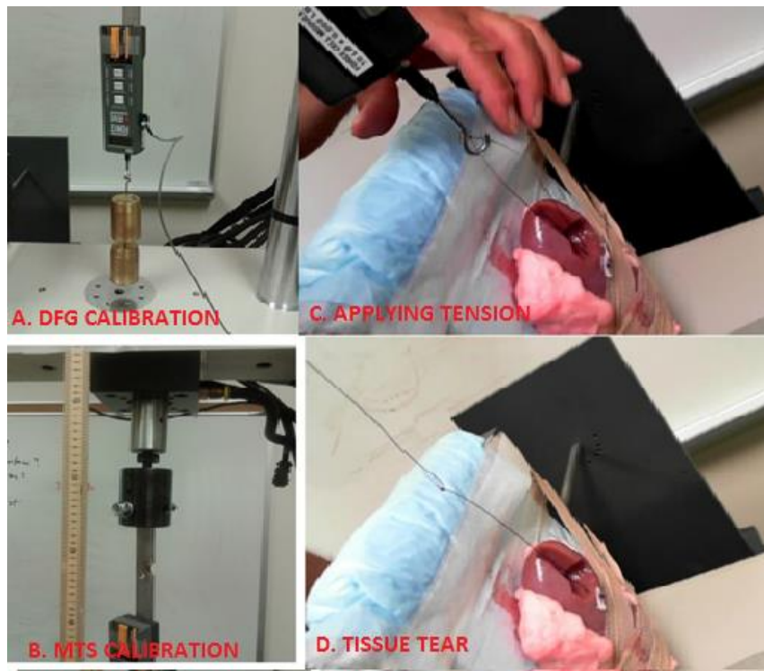
Figure 11: Calibration of DFG and MTS Mini Bionix
