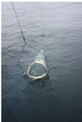
Figure 6 - Ichthyoplankton net showing flow meter inside the net deployed at the buoy site in 46 m of water.
