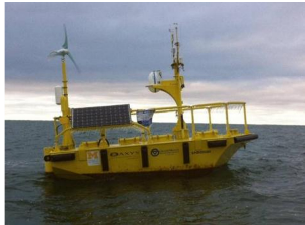
Figure 1 – WindSentinel Floating MET Facility
