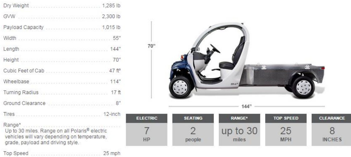
Figure 3-9: Proposed Special Case Vehicle Loading (Polaris Industries 2014)
