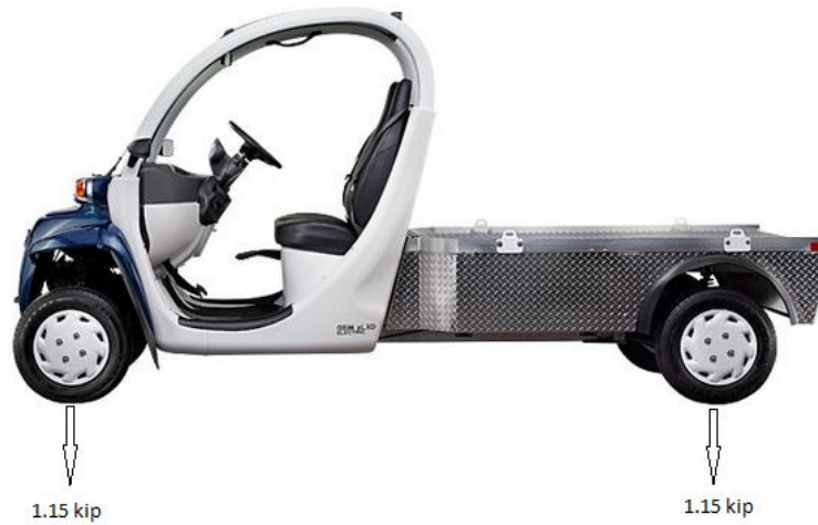
Figure 3-10: Special Case Vehicle Load Configuration (Polaris Industries 2014)
