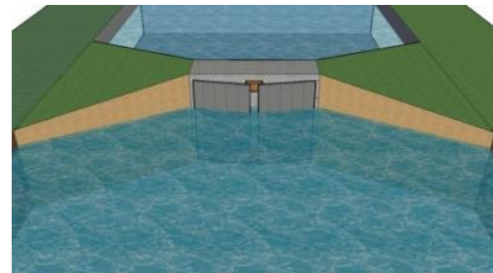
High tide – doors are closed and the fishes blocked
