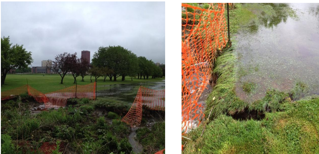
Figure 3.9: View looking east as the flowing stream enters the eroded edge of the site. Gully and rill cracks were observed indicating additional erosion would take place (photo credit: Nathan Frazee).
