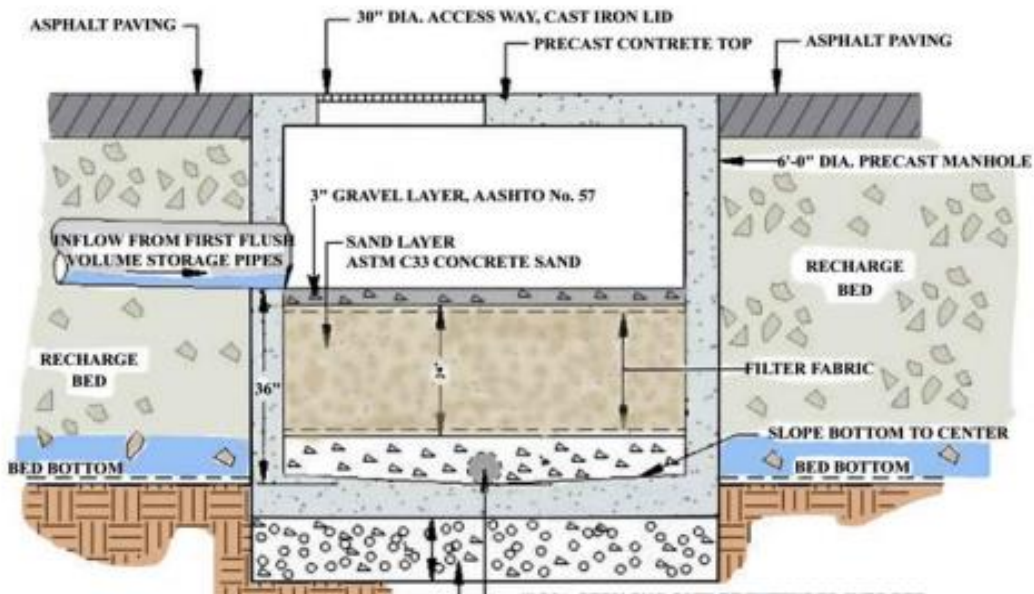
Figure 2.23: Water enters through an inflow pipe, settles through the sand, and exits the structure through a pipe at the bottom (Department of Environmental Protection, 2006).
