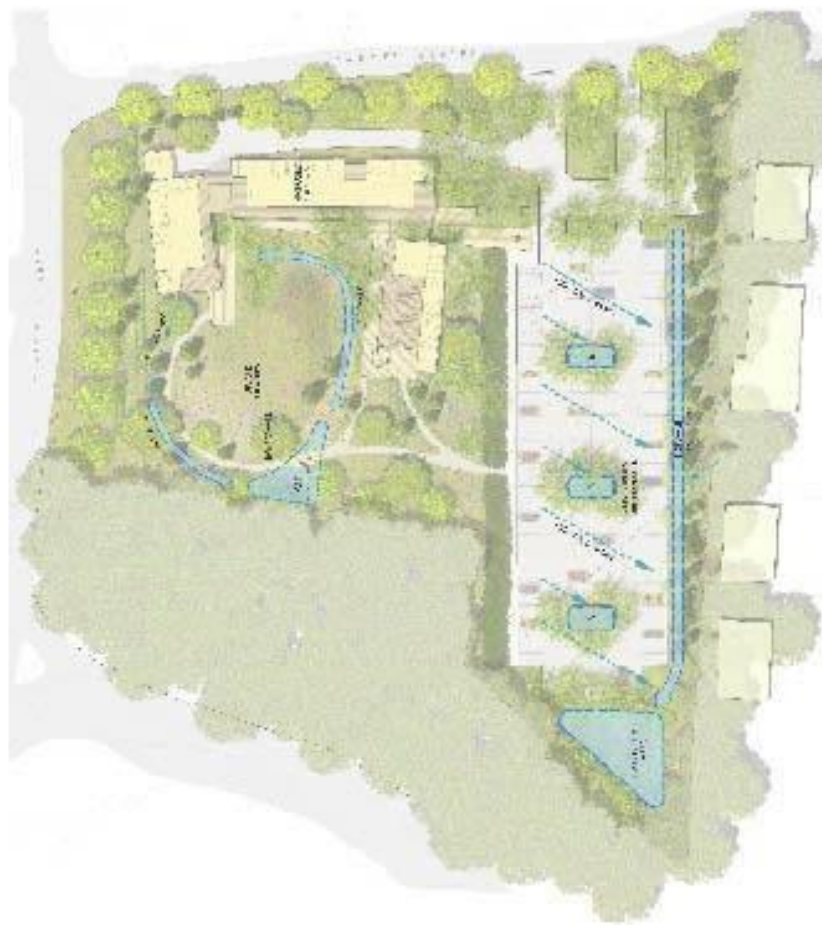
Figure 2.13: Stimson Associates' Low Impact Development project plan, diagram, and sections show swale design and locations (AIA, 2013).
