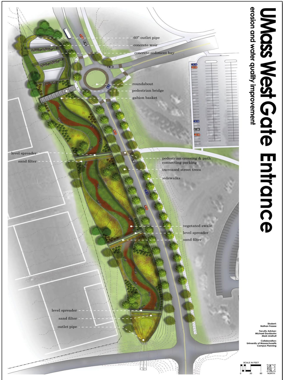
Figure 4.13: The final site plan rendering, showing three large bays with a swale at the bottom and sand filter planting areas
