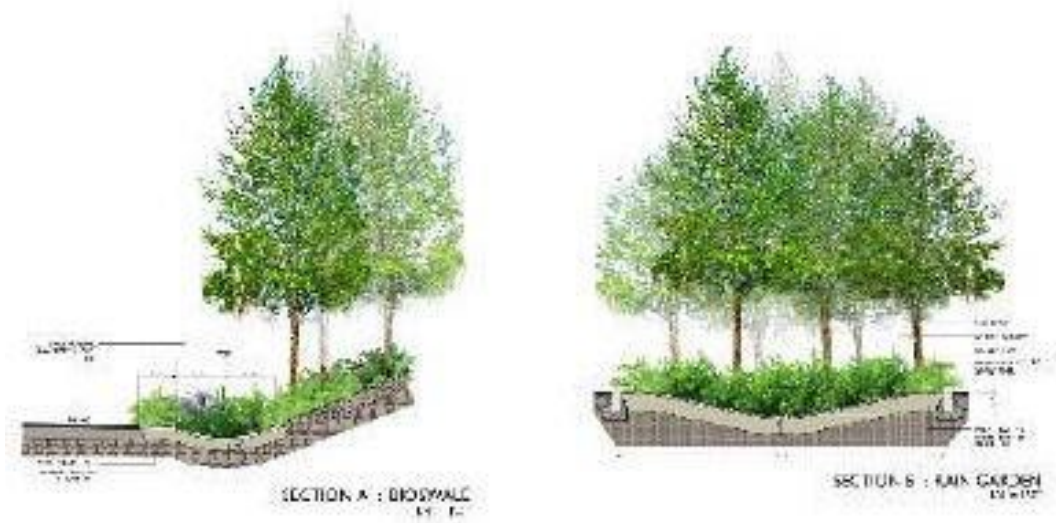
Figure 2.14: Stimson Associates' Low Impact Development project plan, diagram, and sections show swale design and locations (AIA, 2013).
