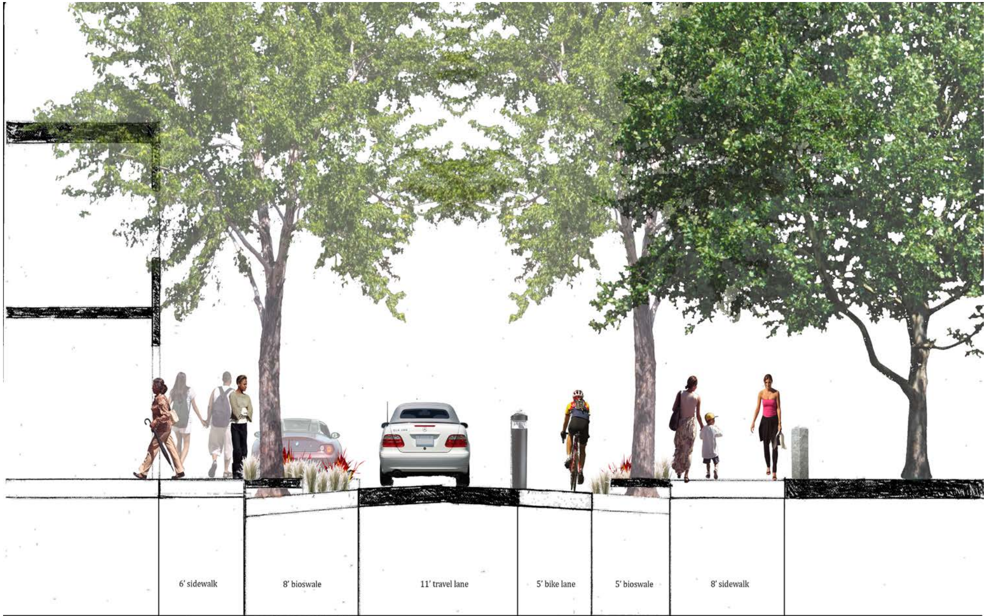
A typical composite section view showing elements of the one way street system. With eleven foot travel lane for vehicles and eight foot parallel parking with bio-swales on either side.
