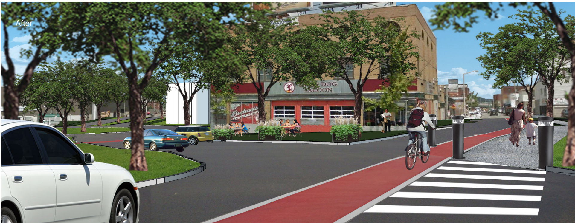
An after image of the previous intersection showing the designed travel lanes for the car as well as pedestrian and bicycle lanes. Bollards at the corner of Water St. keep cars from turning onto the bicycle lane. By narrowing the vehicle lanes and adding large concrete planters for safety an outdoor dining area or beer garden is created in front of the Salty Dog Saloon.
