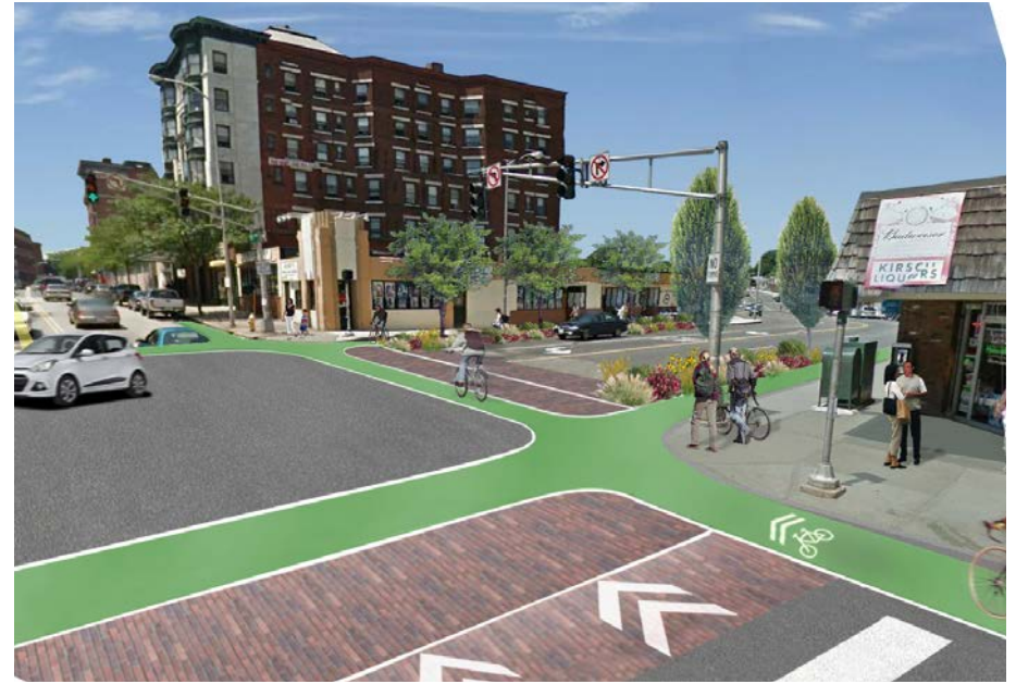
Figure 9: This rendering shows the raised pedestrian table that facilitates pedestrian movement across wide intersections.
