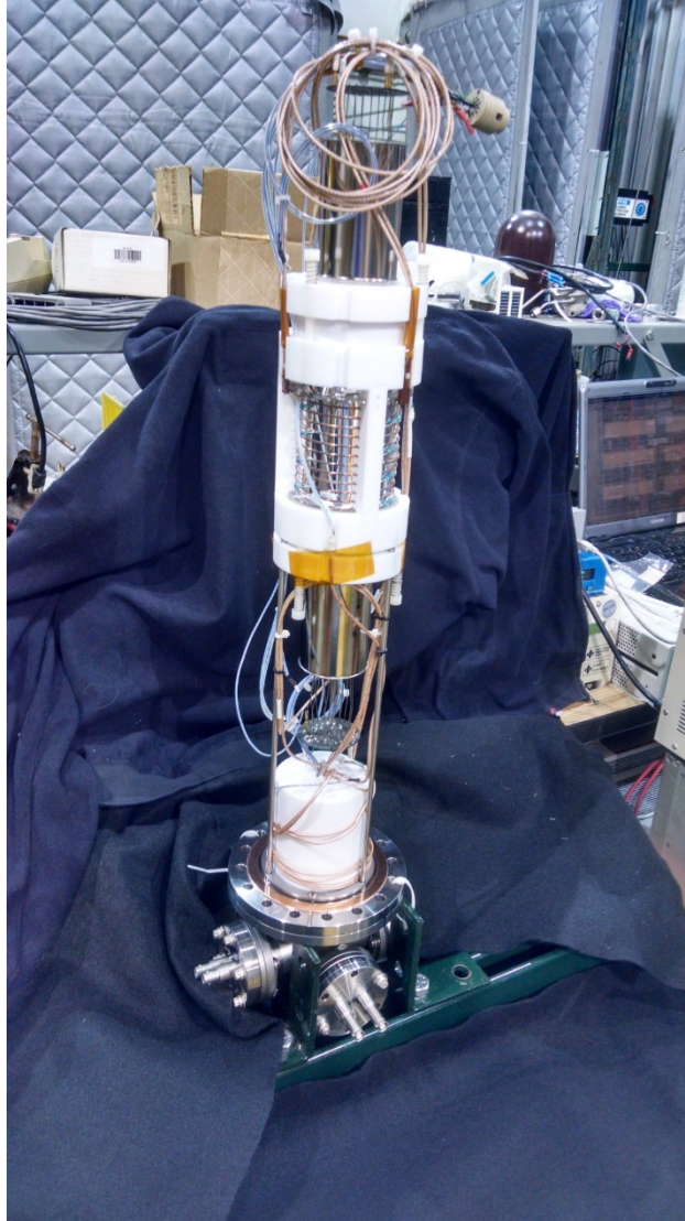
Figure 3.2: The TPC with PMTs and level and temperature monitoring hardware as prepared for this campaign. As compared to previous campaigns with the SCENE Detector, a PTFE cylinder was added to the base of the detector volume to reduce the amount of argon required to fill, with the security of the Underground Argon in mind. Otherwise, the setup remains the same as previous, published campaigns.
