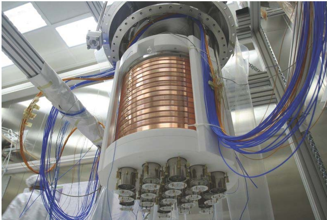
Figure 1.2: Reproduced from[5]. The DarkSide-50 TPC.
