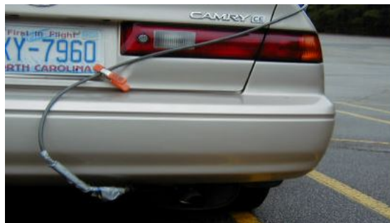
(b) Sampling probe that measures tailpipe emissions
