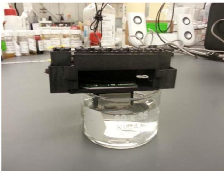
3. Place beaker into the sonicator. Turn on the sonicator for a few minutes depending on how much impurity comes out.
