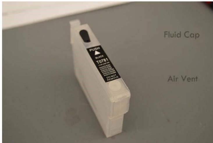
2. Open the fluid cap of the cartridge and place the cartridge on a bench (with a paper towel underneath in case of a spill).
