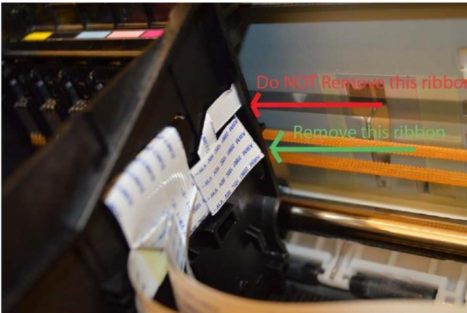
12. You need to remove the pin connector. Using the small tipped screwdriver, press on the hole shown below. While you are pressing on this hole, pull firmly up on the pin connector. The pin connector will eventually loosen if you hit the spot correctly. You will eventually get it but it will require a lot of patience.
