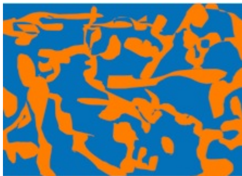
Figure 1.1: Representation of the bulk heterojunction morphology meeting the requirements for interface and percolation of two component functional materials.
