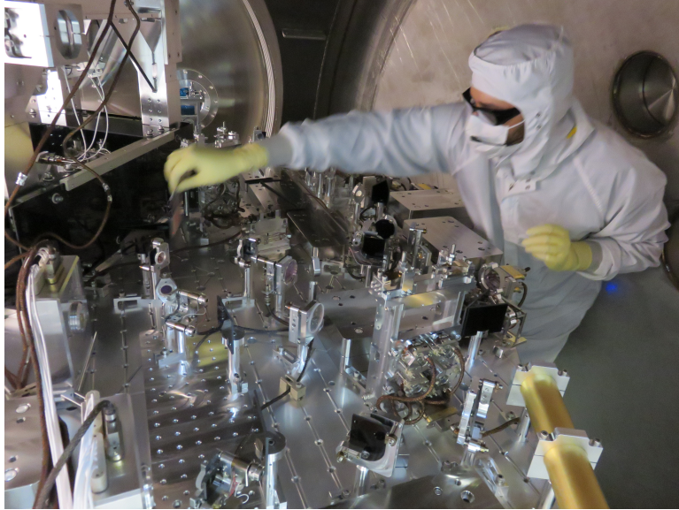
Figure 6.13. Photo of the author working to check beam alignment into the OMC black glass shroud, designed to enclose the output mode cleaner in a non-reflective covering to prevent scattered light. The black welder's glass can be seen around the OMC suspension cage in the upper left of the image.
