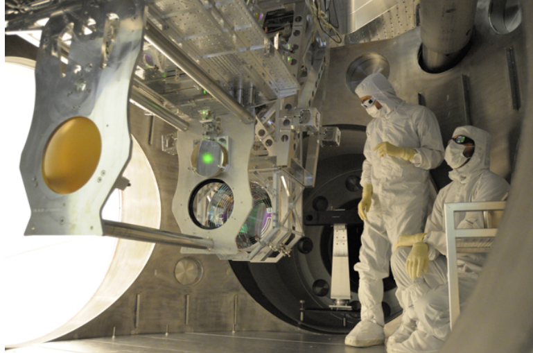
Figure 5.3. Photo of the author in the ETMY vacuum chamber, working on alignment of the green laser. I am kneeling, Keita Kawabe is standing.
