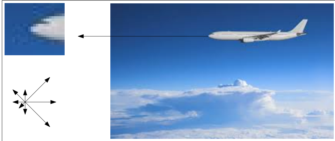
Figure 3.5. An illustration of gradient orientation distributions of the nose of an airplane.
