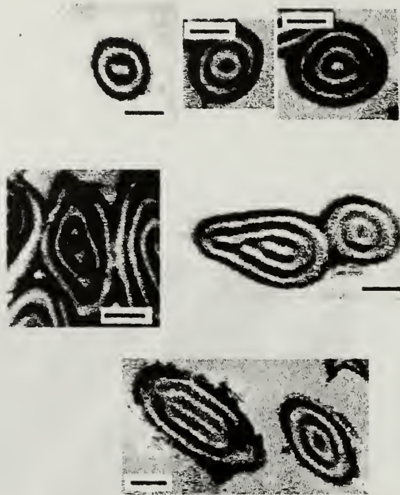
Figure 3.7. TEM images of bulk lamellar-forming PS- b -PBD structures in pores of various diameter. Scale bars: 100 nm. 9
