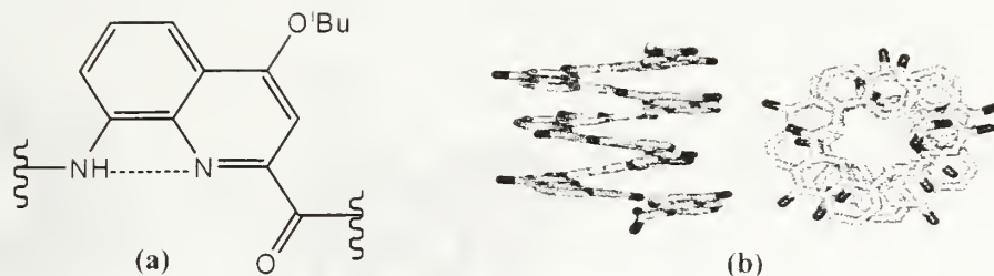
Figure 1.4: (a) Aromatic \delta -peptide with quinoline backbone. (b) Side and top view of crystal structure. Side chains, solvent molecules, and hydrogens were omitted for clarity. Reported structure has 8 repeat units forming a helix with just over 3 turns. Taken from reference (25).
