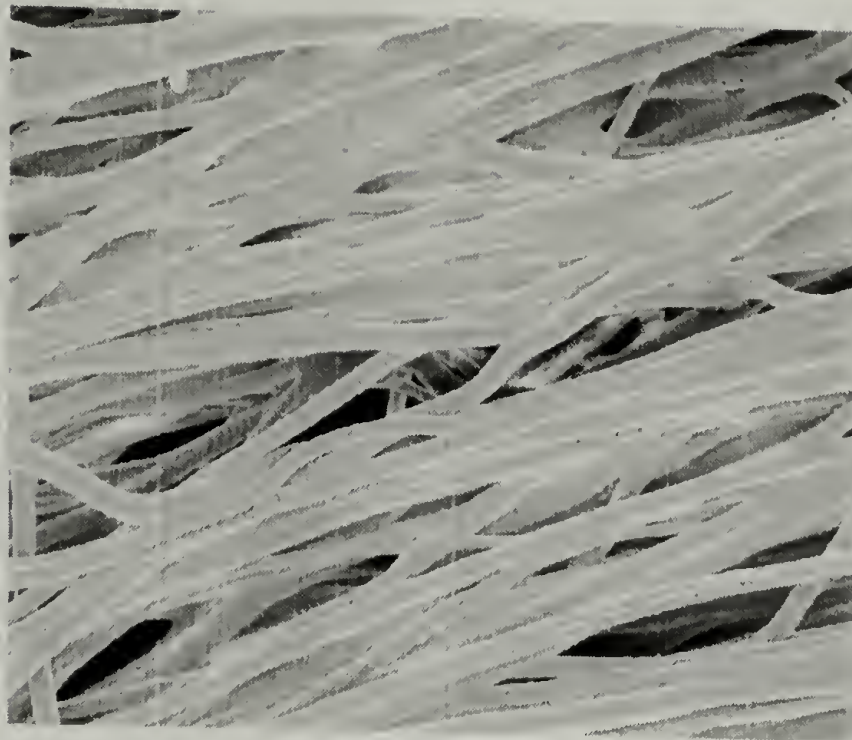
Figure 2.18 – Electrospun Pellethane® 2103-80AE; collected onto a target rotating at 9.84 m/s.
