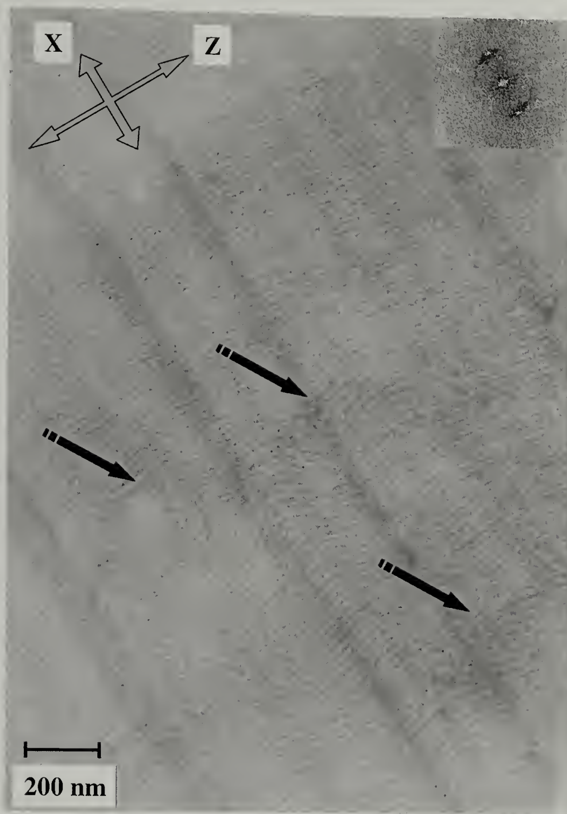
Figure 7.6 Cross-sectional TEM image of typical defects. While there were few defects, the defects shown were observed the most frequently.
