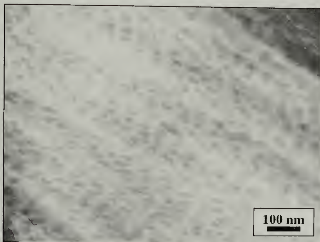
Figure 4.8 PS- b -P4VP copolymer stained with iodine
