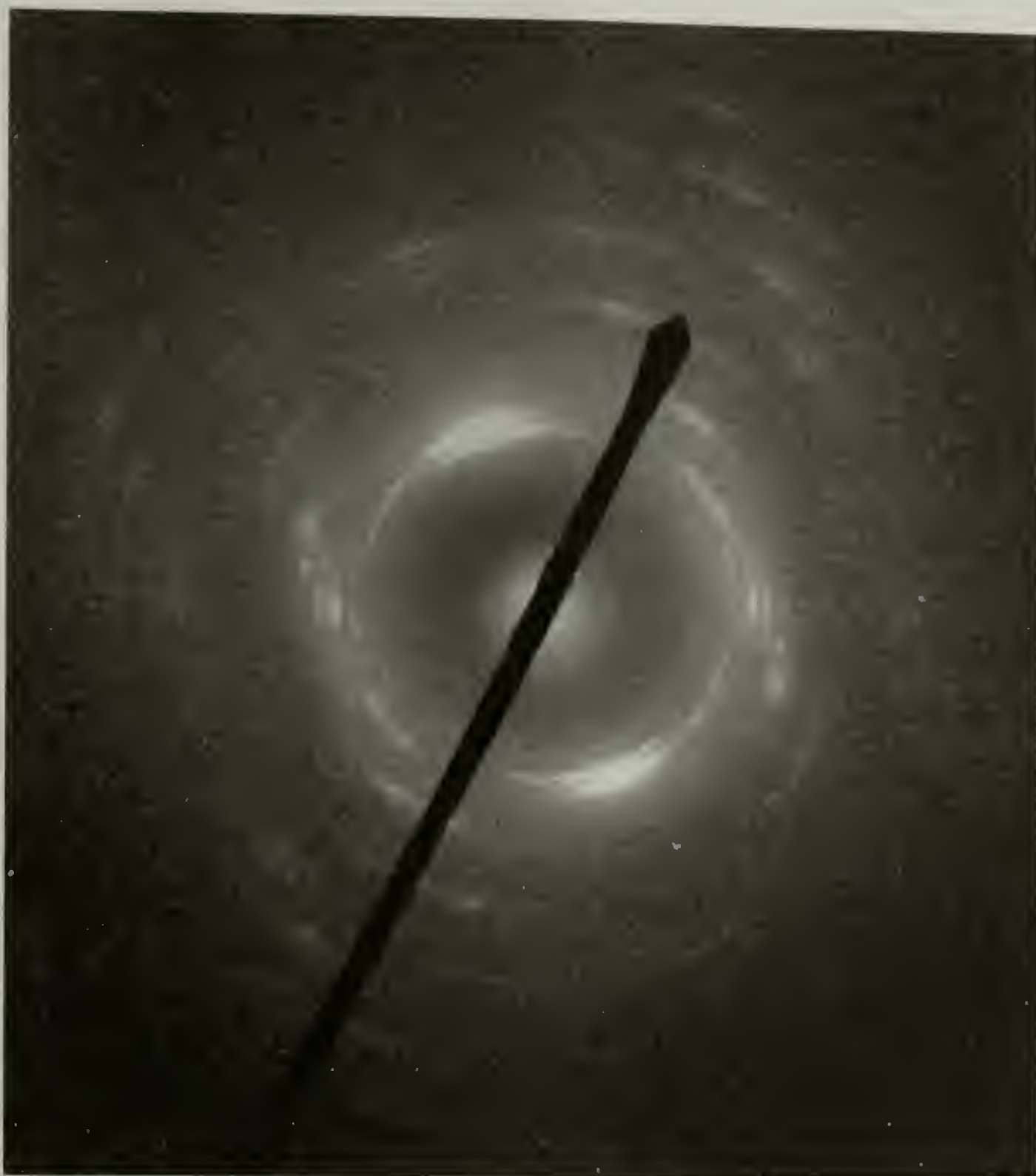
Figure 59: Diffraction pattern from a spongy region of a fibroin film prepared at the 5% aqueous fibroin-hexane interface.
