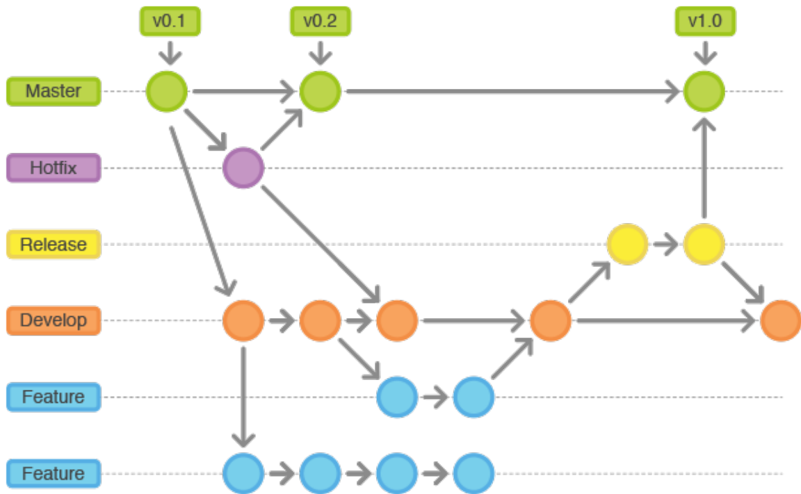
Figure 7. Example of a Github Workflow
