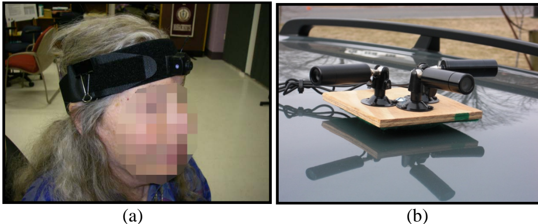
Figure 1. Field drive camera system. (a) You will be wearing a lightweight, wireless headband camera. (b) We will install three cameras on the roof of your car with a felted, industrial strength magnet to prevent scratching or movement.
