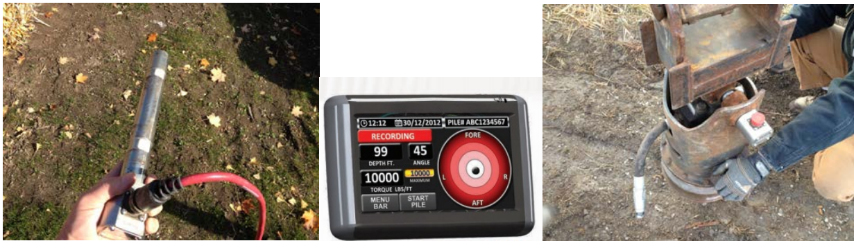
Figure 4.13 TORQ-PIN, 4.3" LED TORQ-PIN Display, TORQ-PIN Installation (from left to right).
