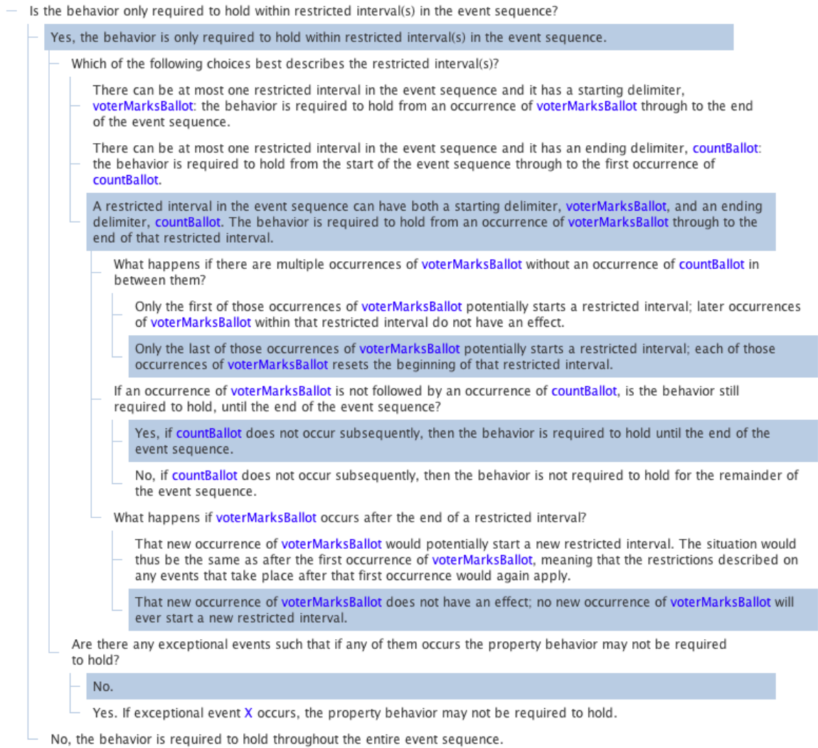
Figure F.1. Scope question tree for the property “After a voter marks ballot event, no insider marks ballot event can occur until count ballots occurs.”
