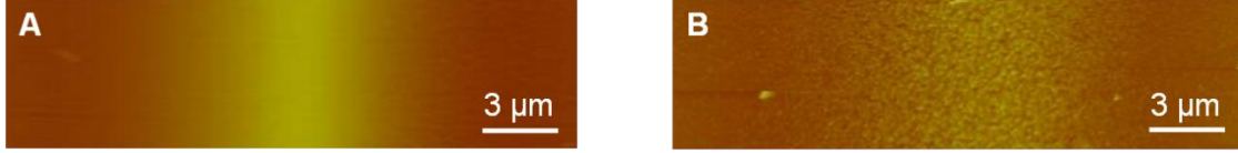
Figure 3.10 – AFM height images of a line in the nanocomposite. (A) Before the 450 °C heating. (B) After the 450 °C heating.
