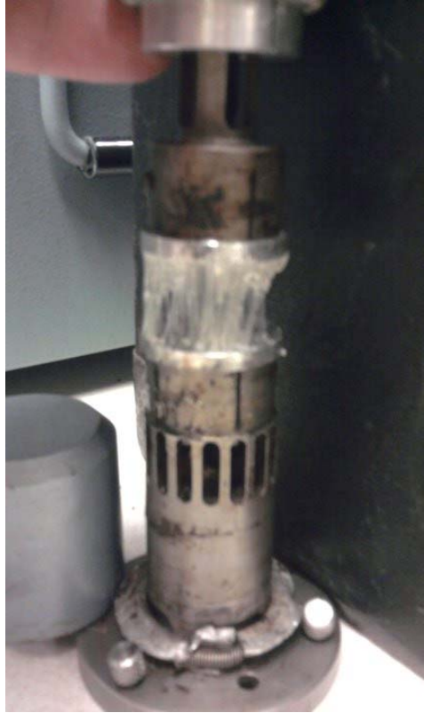
Figure 1.5 - An example of fibril formation of an adhesive adhered between two plates of a parallel-plate rheometer.
