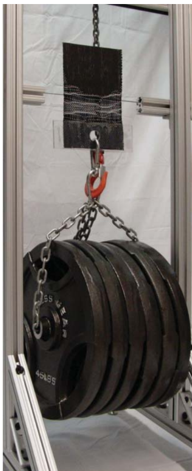
Figure 1.9 - A 100 cm 2 adhesive pad supporting 130 kg of load. Used with Permission: Adv. Mater. 2012. 74
