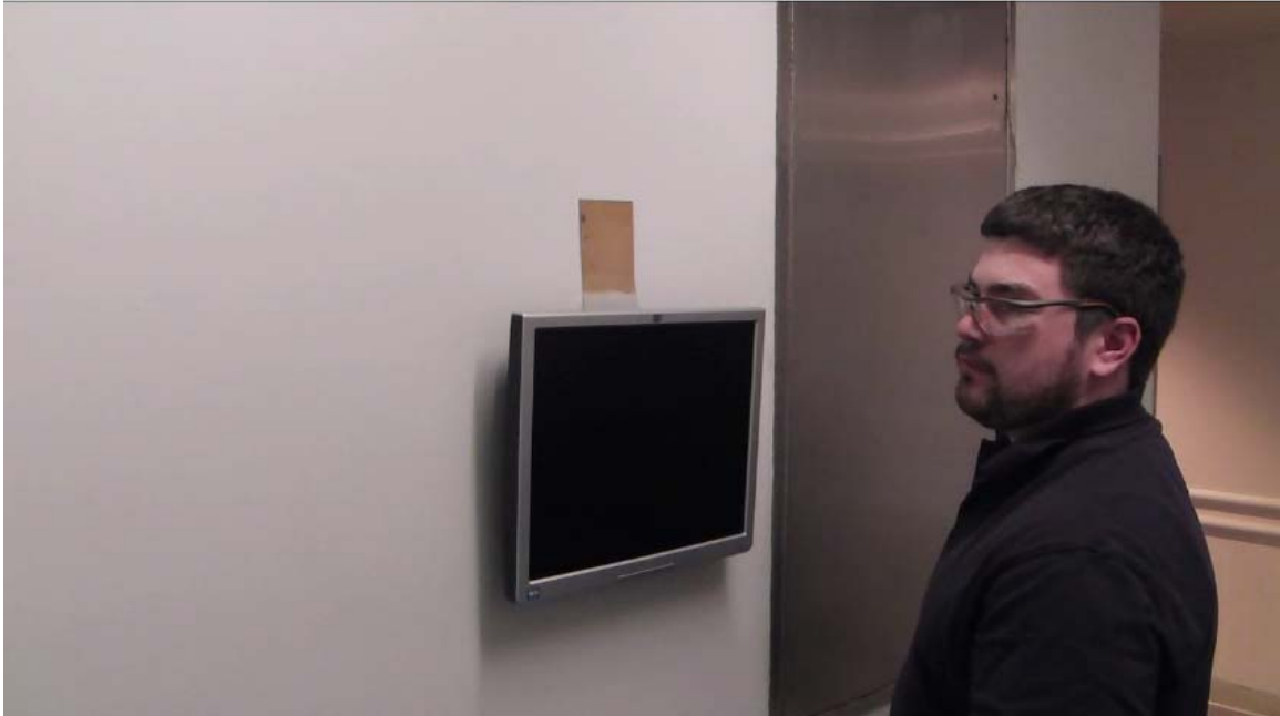
Figure 3.11 - Photograph of a LCD computer monitor hanging on drywall with a gecko-inspired adhesive. Adhesive consists of glass fiber fabric and PU-C.
