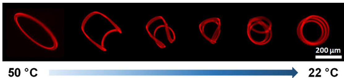
Figure 5.5 Thermal actuation of a circular ring ( a = 190 \mu\text{m} ) of photo-patterned PNIPAM hydrogel. Upon swelling as the temperature is reduced from 50 to 22 °C, the ring adopts characteristic shapes corresponding to values of O increasing from 1 to \approx 3 .
