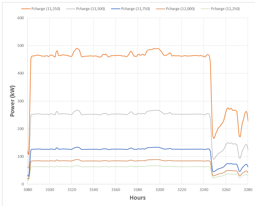
Figure 3.5 Comparison of Charging Pump Power Consumption (200 hour period)
