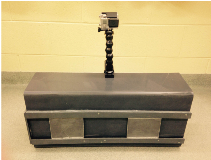
Figure 2: Testing apparatus with GoPro camera attached
