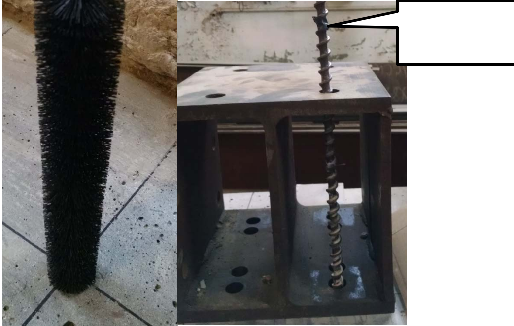
Figure 8.6 Brush Cleaning Hole (Left) and Alignment guide for Test Series 0b an 0c (Right)
