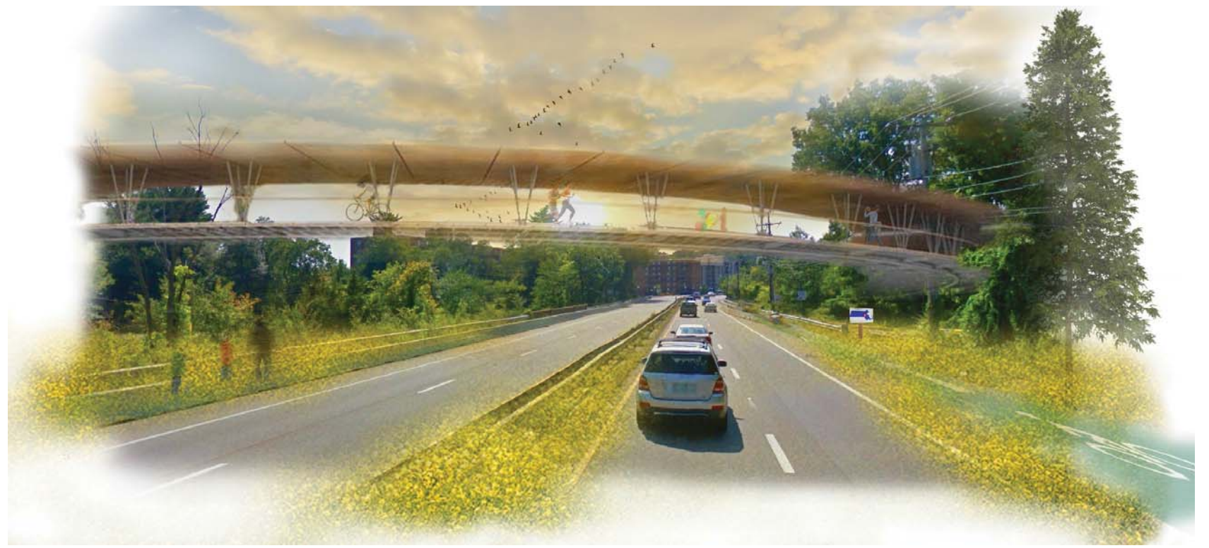
The wood timber and steel bridge proposal get pedestrians and bicyclists over Route 9 in a safe and efficient manner along the greenway. The structure is a looping ramp that is ADA accessible. It increases connectivity of south Framingham and north Framingham.
