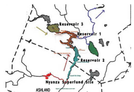
The image below illustrates the directions of water flow throughout the reservoir systems. Reservoir 3 and the Sudbury river flow southeast, linking into reservoir 1. Reservoir 2 is fed by the water systems in Ashland that are contaminated with Nyanza. From reservoir 1, the water combines and flow through the Sudbury
