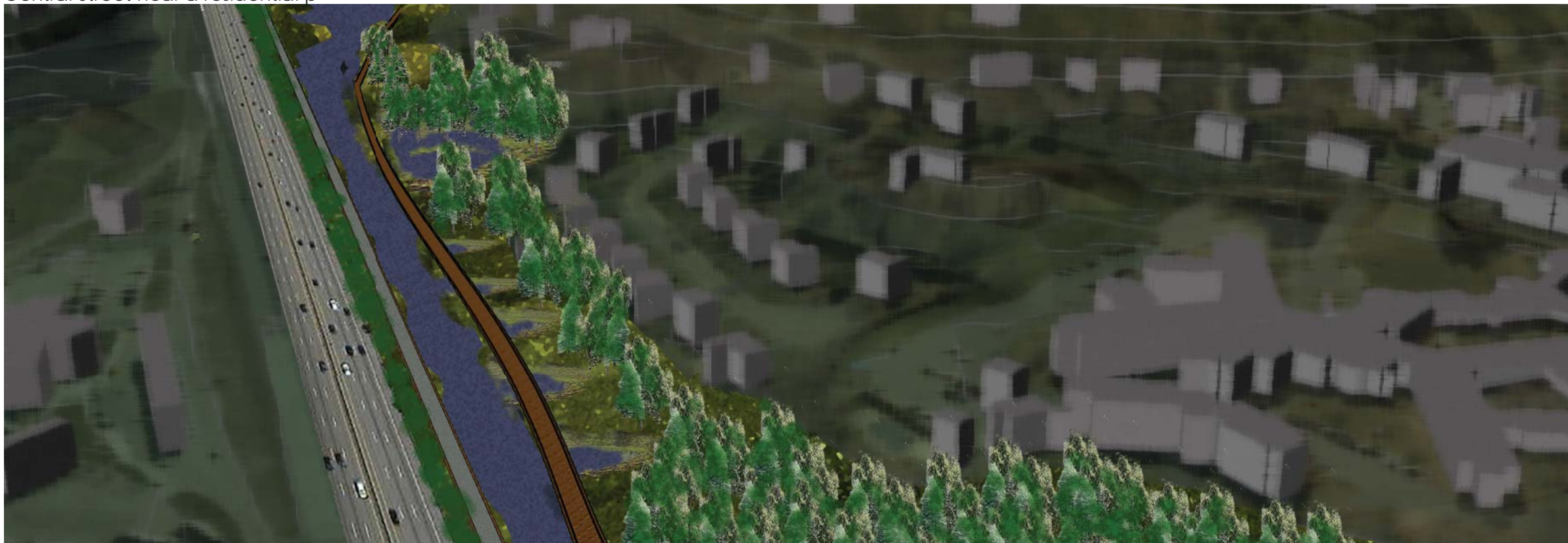
Focus Area: This is located by the Simpson Park. The boardwalk is designed to be able to sit on grade, or float on the water when water elevation rises. The boardwalks also turn into paths when they go on a grade that will not usually flood. This area is also located close to Central Street near a residential p
