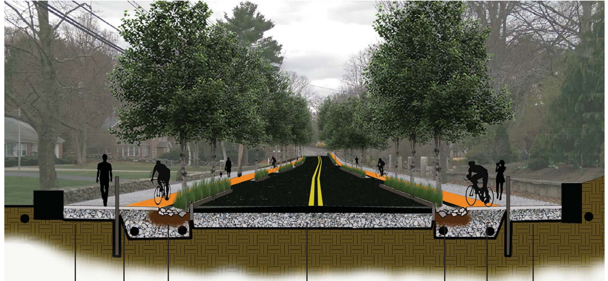
Sidewalk Bike lane BioSwale Central Street BioSwale Bike lane Sidewalk Central Street after: In order to protect the Sudbury from more pollution the streets should be a pervious surface, this section bike lanes, sidewalks and the streets are a pervious paving with the addition of bioswales
