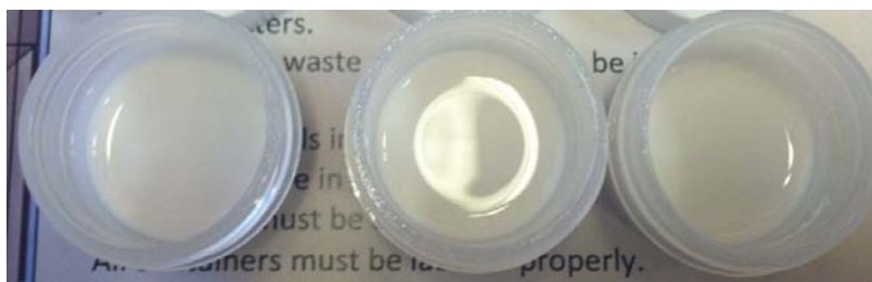
Figure 4-3 Titania particle (Sun Innovations, Inc. Anatase phase, 5-10 nm, >99%) surface modification with (a) D 4 , (b) trimethylsiloxy-terminated polydimethylsiloxane (M w ~2000) and (c) D 4 H . Vapor phase reactions were carried out by adding 0.5 g silane or silicone to ~ 1.0 g titania particles, followed by heating the mixture at 150 °C for 3 days within a sealed vessel.
