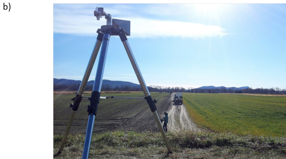
Figure 3.12. a) Schematic showing the experimental setup to make measurements of antenna patterns using horn antenna. The phase center of PTWR antenna array is at O , and a horn antenna at H . b) Horn antenna was mounted on a tripod located at the Connecticut River Dike Path in Hadley, MA.
