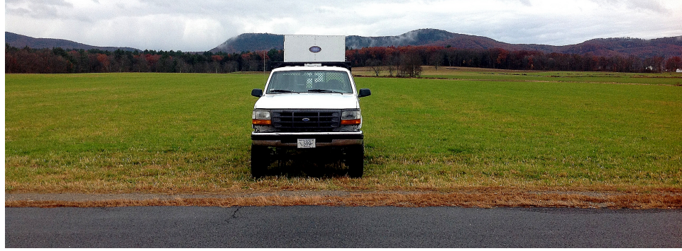
Figure 4.17. Radar deployment on 11/07/2013. Holyoke Range was chosen as a clutter target in order to provide high signal to noise ratio.
