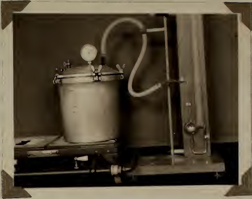
Plate II. Apparatus for determining pressure developed in glass jars during processing in a pressure cooker
