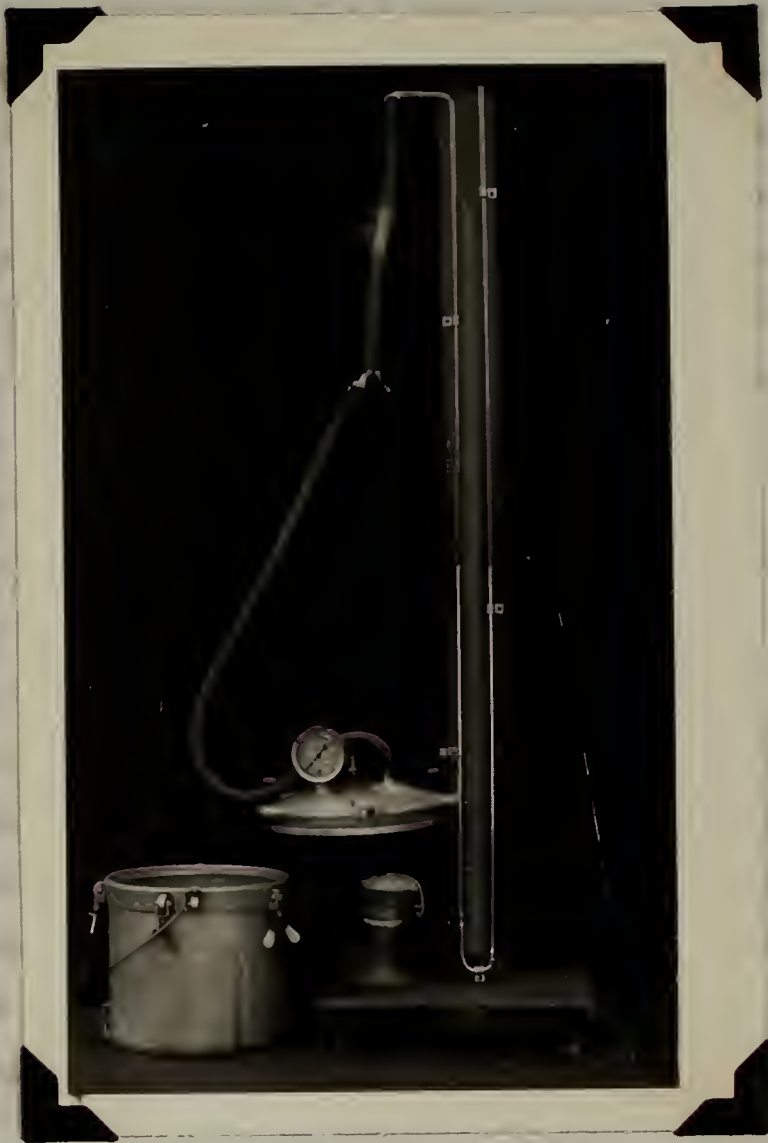
Plate IV. Apparatus for the determination of internal pressures.
