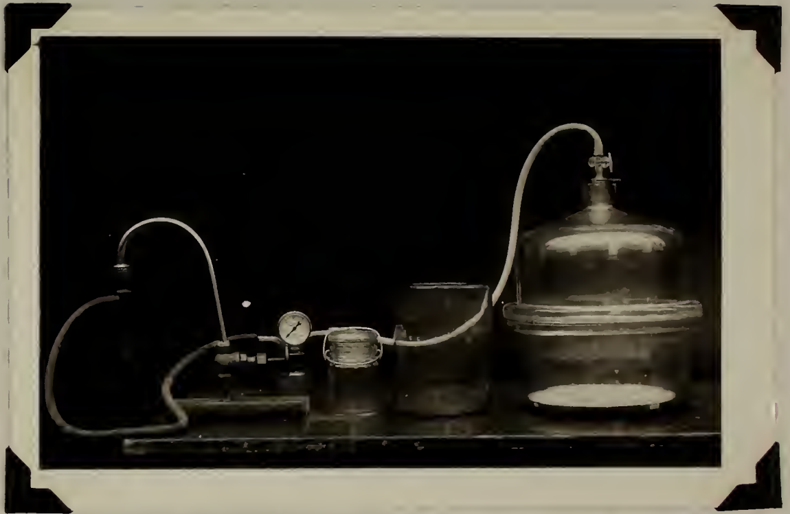
Plate VI. Apparatus for the determination of vacuums by the vacuum desiccator method.
