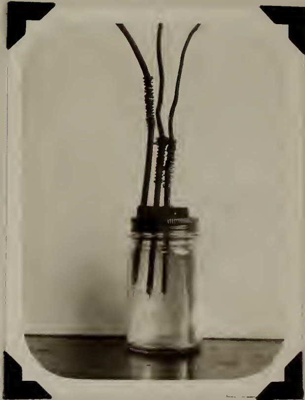
Plate 5. Apparatus used for determining the temperature in various parts of the jar.
