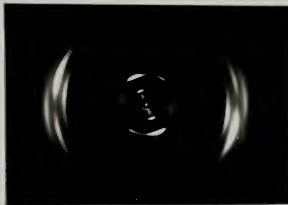
Figure 2.11 WAXS patterns of a 2,4-LCPU-6 [\eta]=0.60 dL/g fiber, drawn from the melt (A), soxhlet extracted in hot MeOH for 5 days (B), and annealed at 165 °C for 5 more days (C). Fiber axis is oriented vertically.
