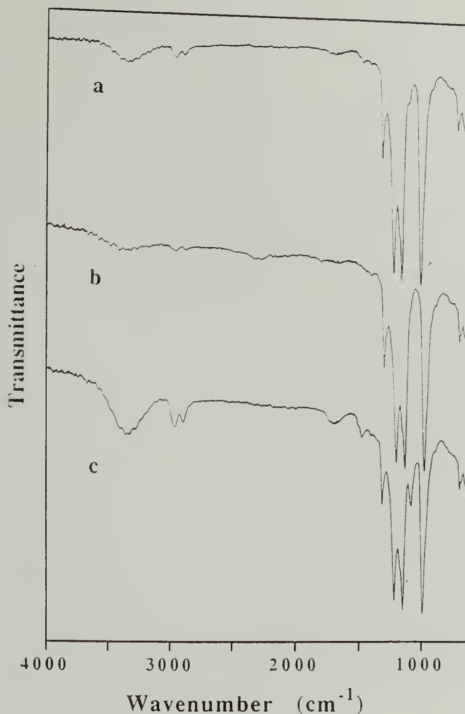
Figure 3.9. ATR-IR spectra of the hydrolysis product of PCTFE-PEAA (-15 °C) as a function of solvent composition (methanol:water): (a) (100:0), (b) (50:50) and (c) (0:100).
