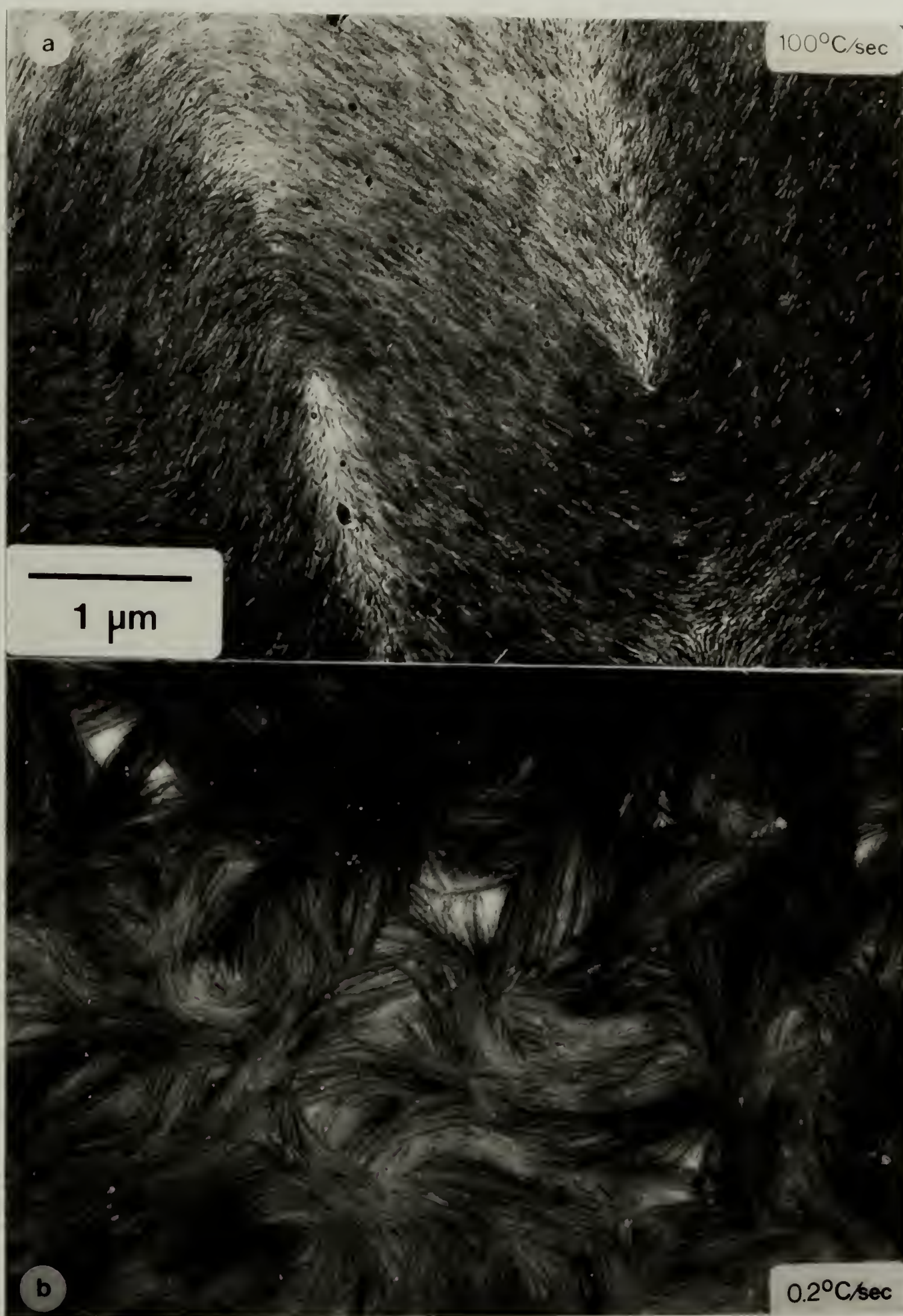
Figure 2.11 Morphology of TQT10-M for (a) rapid (100°C/sec) and (b) slow (0.2°C/sec) cooled samples. The lamellae in (b) are thicker and larger than those in (a). The lack of spherulites in (b) may be due to a high defect density in the precursor nematic, or perhaps TQT10-M is less likely to form spherulites than OT06 shown in figure 2.12. See text for sample preparation.
