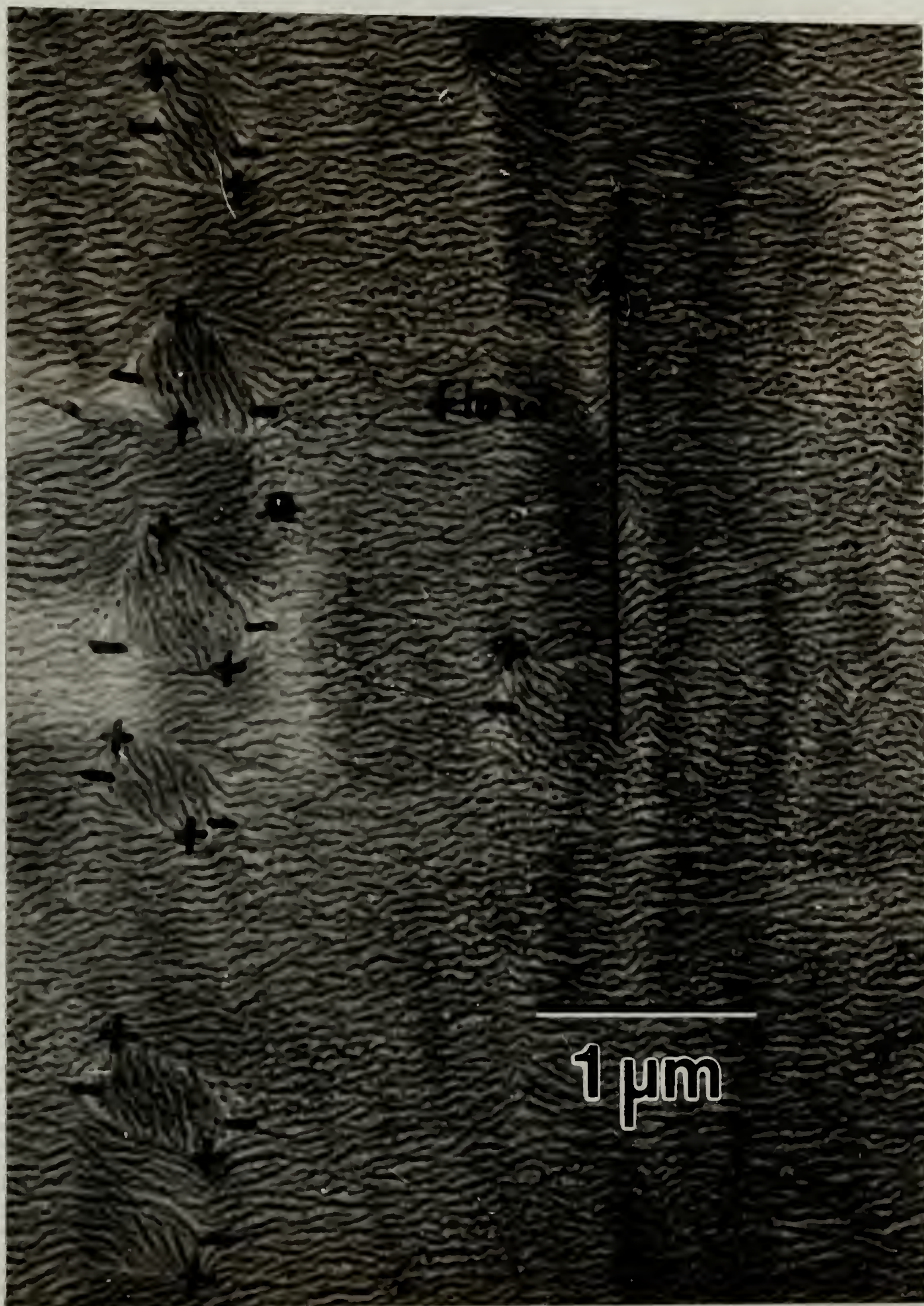
Figure 6.11 The Lehmann cluster observed when \xi \sim d . (b) Extensional flow oriented sample from Wood [1985]. (Continued next page.)
