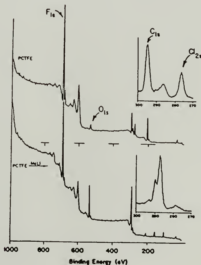
Figure 1-3-4. XP spectra of PCTFE film and PCTFE film after reaction with Methyllithium.
