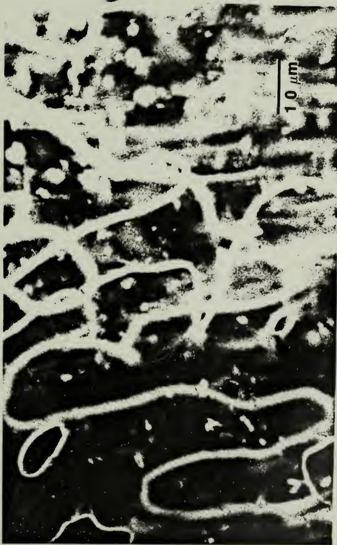
Figure 21: Schlieren texture in 9% PBT in MSA after 48 hours relaxation.
