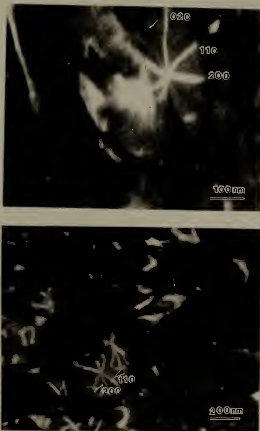
Figure 2.8 (a) annular DF STEM image of PE lamella (b) 110/200 annular DF STEM of PE thin film illustrating (100) lamellae in reverse contrast (dark lines). Bend contours are labelled consistent with lamellar growth direction.
