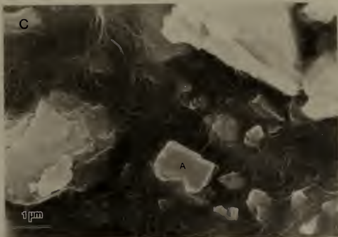
Figure 3.13 c) SEM-SEI image of duPont PE/CaCO 3 composite.
