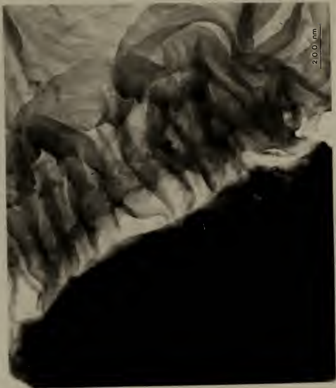
Figure 3.8 BF CTEM of duPont PE/CaCO 3 interface at high magnification.
