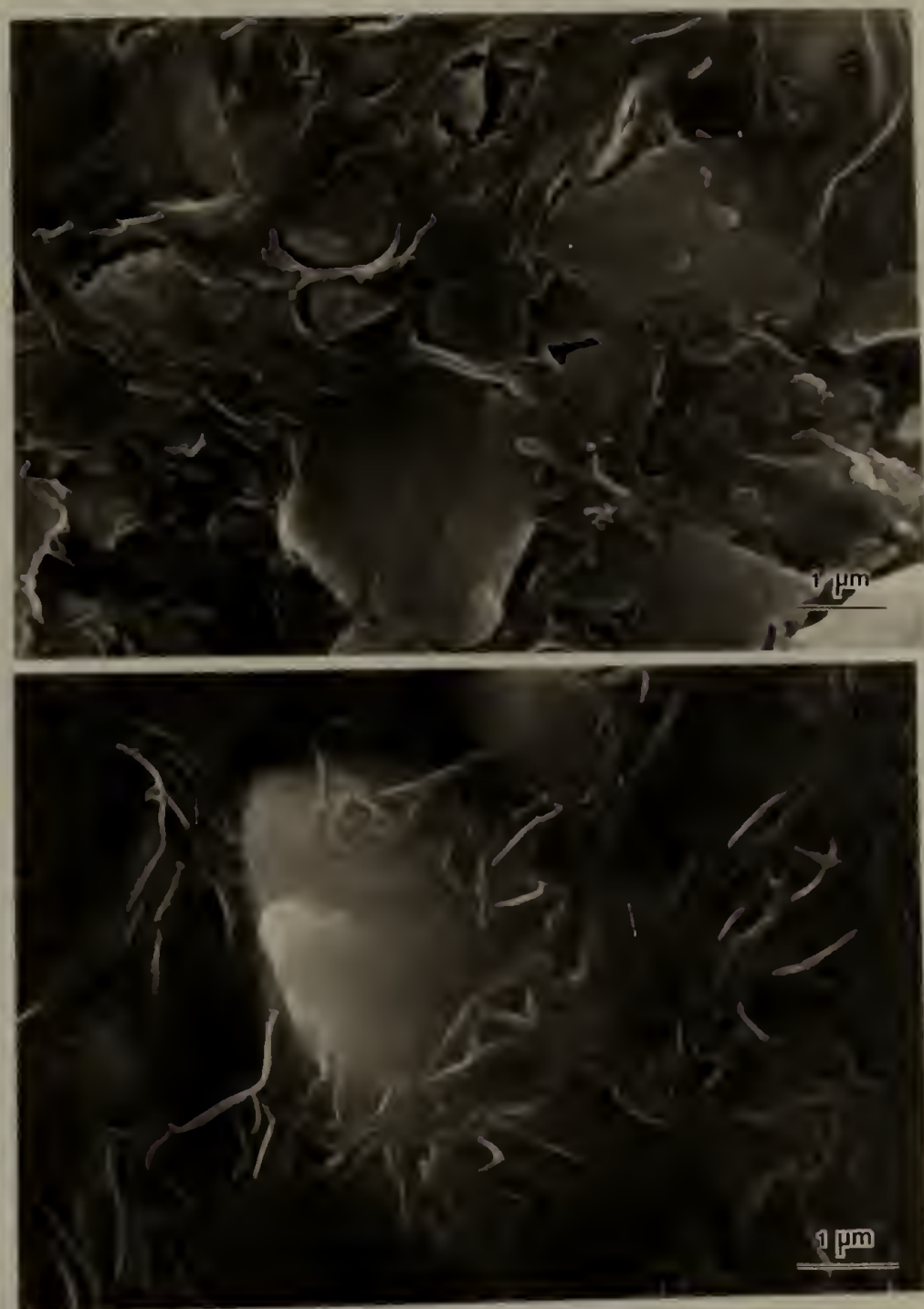
Figure 3.13 SEM-SEI images of filled polyethylenes a) Alathon®/40% treated CaCO 3 and b) Marlex®/40% treated CaCO 3 .
