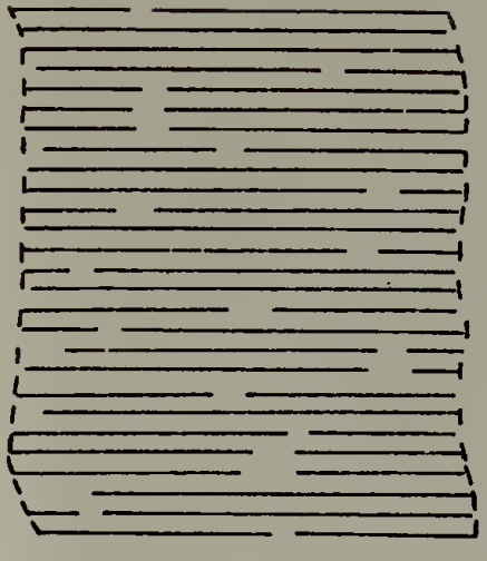
b. Extended Chain Model For The Inner Core Of The Instron Strands
