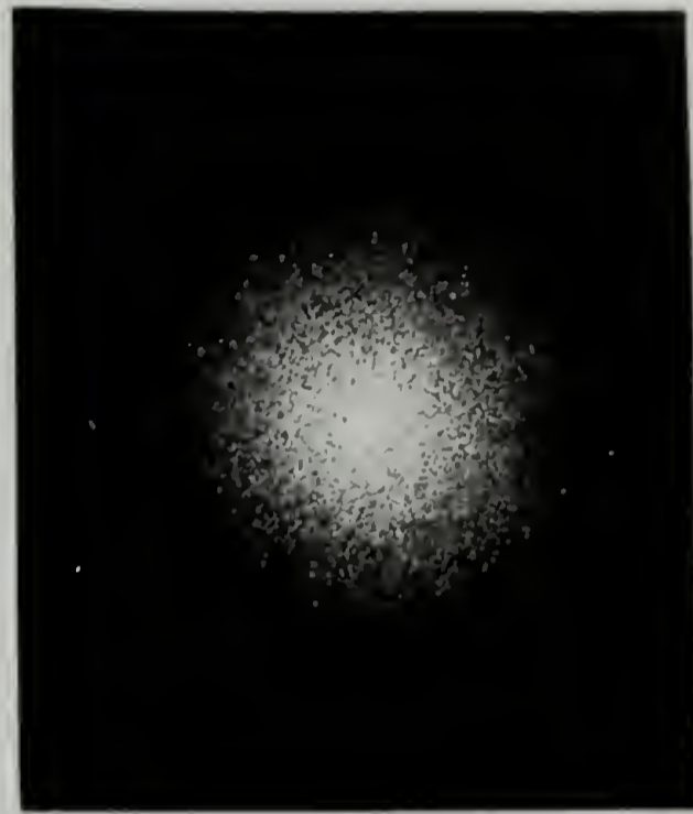
FIG. IVC-14. HV LIGHT SCATTERING PATTERNS FOR 3.0 MIL CHOLESTERYL MYRISTATE SAMPLE AT 81°C. AT DIFFERENT TIME INTERVALS.
