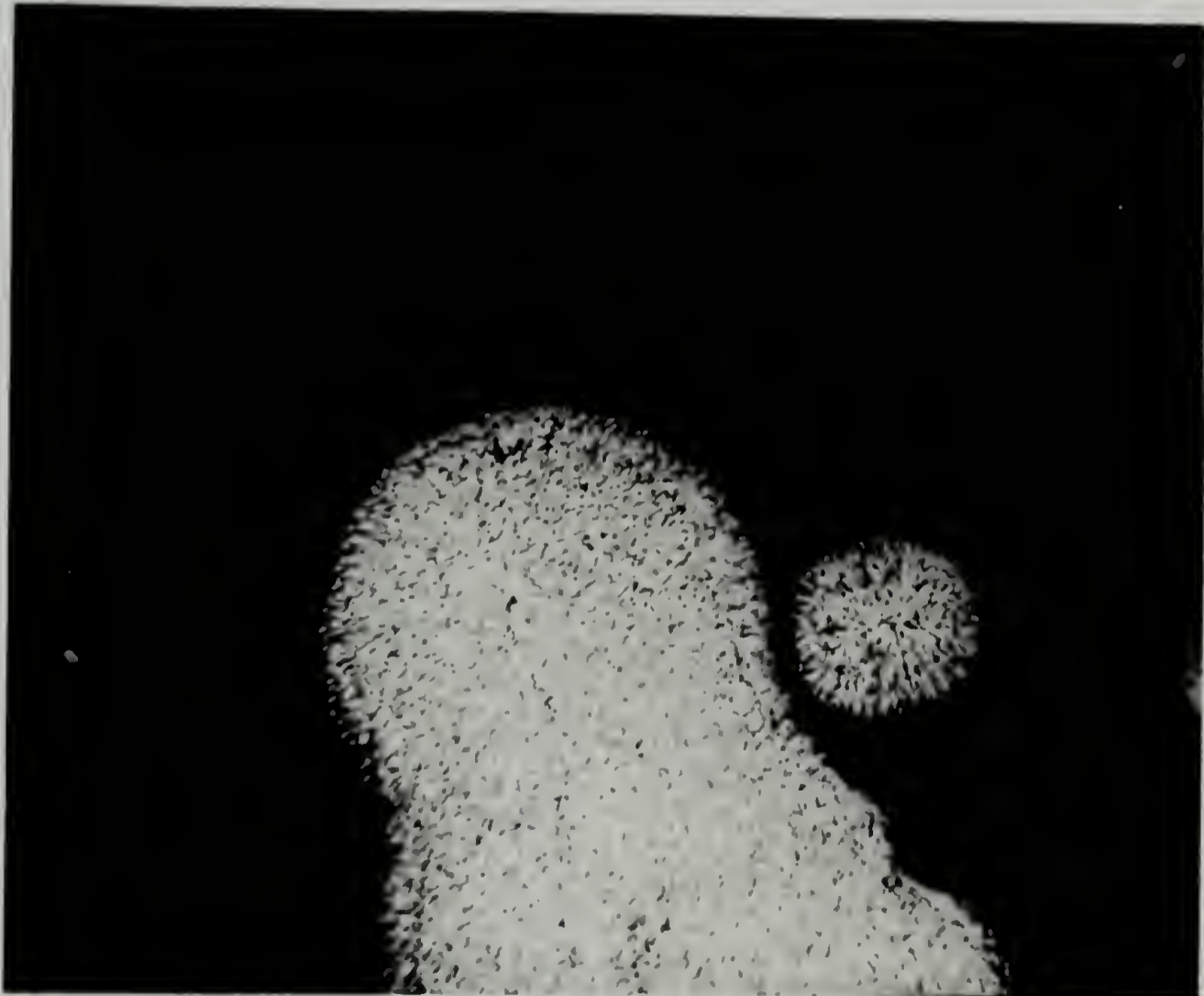
FIG. IVC-13. PHOTOMICROGRAPHS OF 3.0 MIL CHOLESTERYL MYRISTATE SAMPLE AT 81°C. AT 22 MINUTES (left) AND 30 MINUTES (right). \sim 80 \mu
