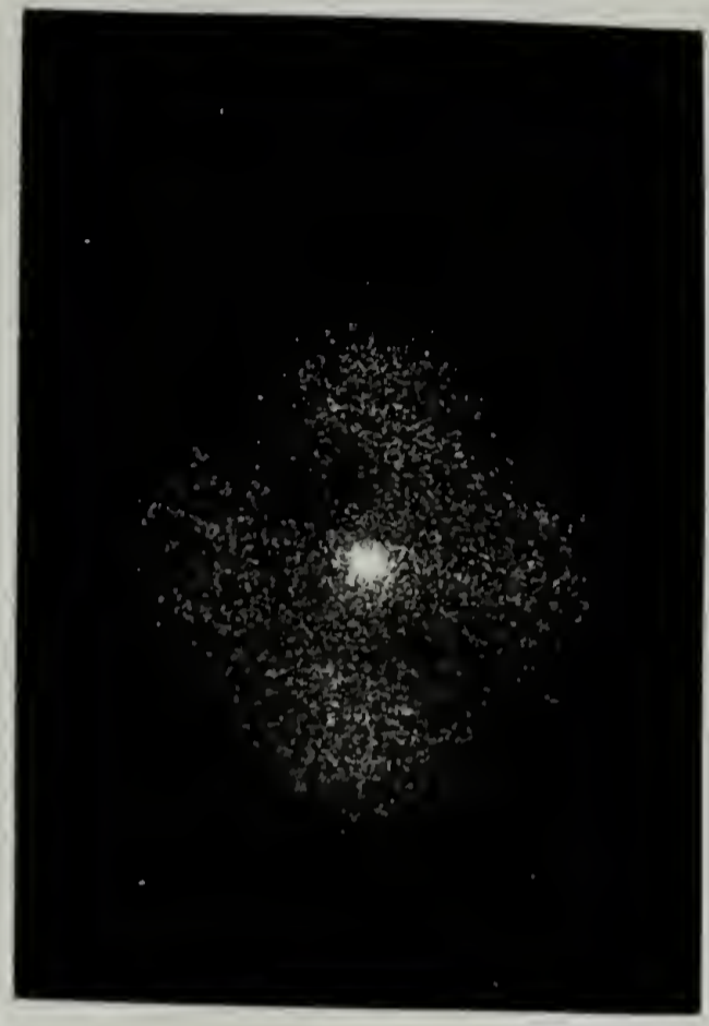
FIG. IVC-1b. Hv LIGHT SCATTERING PATTERNS OF 0.5 MIL CHOLESTERYL MYRISTATE SAMPLE AT 80°C AT DIFFERENT TIME INTERVALS.
