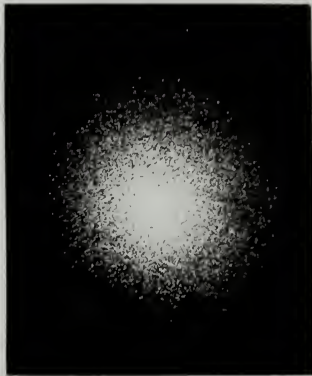
FIG. IVC-14. HV LIGHT SCATTERING PATTERNS FOR 3.0 MIL CHOLESTERYL MYRISTATE SAMPLE AT 81°C. AT DIFFERENT TIME INTERVALS.
