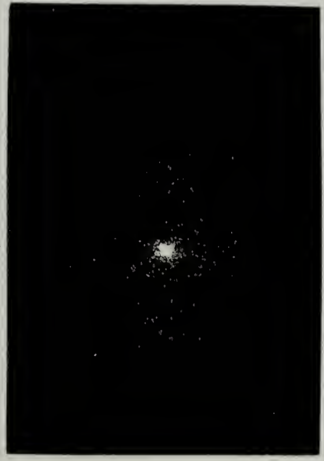
FIG. IVC-1b. Hv LIGHT SCATTERING PATTERNS OF 0.5 MIL CHOLESTERYL MYRISTATE SAMPLE AT 80°C AT DIFFERENT TIME INTERVALS.
