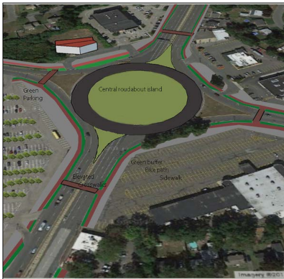
Figure 15 New roundabout design in Northern Rotary
