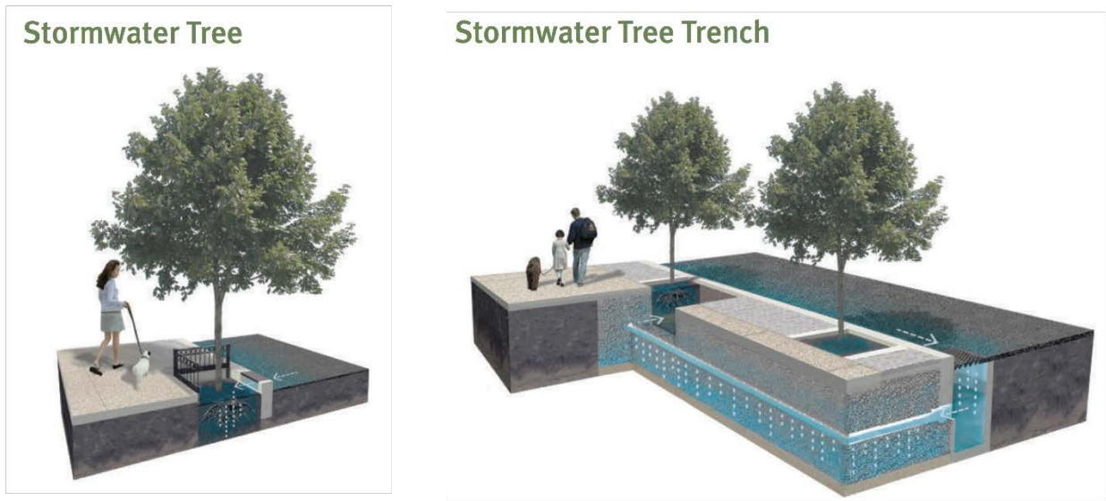
Figure 36: Storm-water Trees and Trenches
