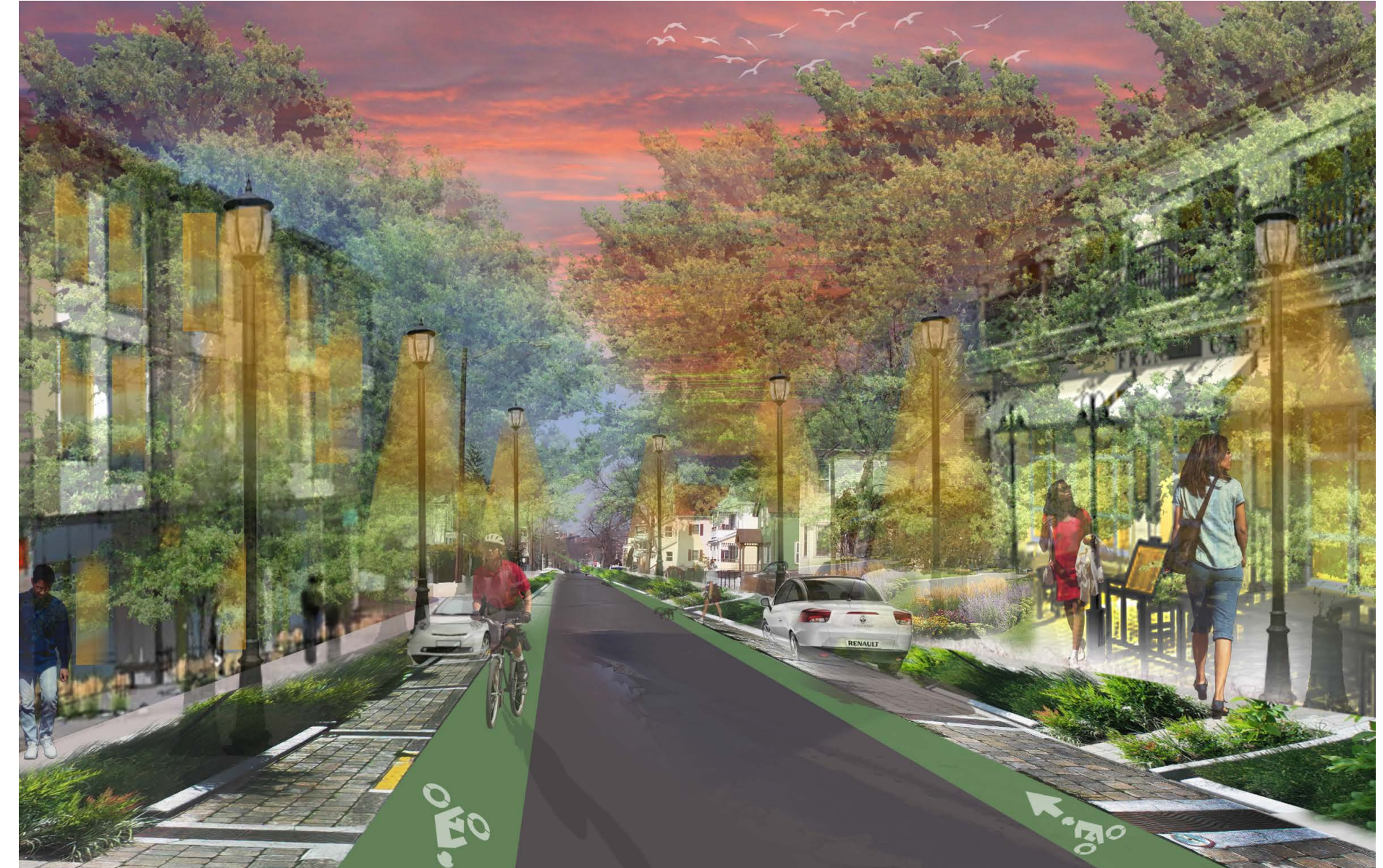
A completed scenario of Massasoit Street with green infrastructure interventions: Infiltration strips, permeable paving in the parallel parking spaces, two-way bike lanes, tree plantings, and street lighting.
