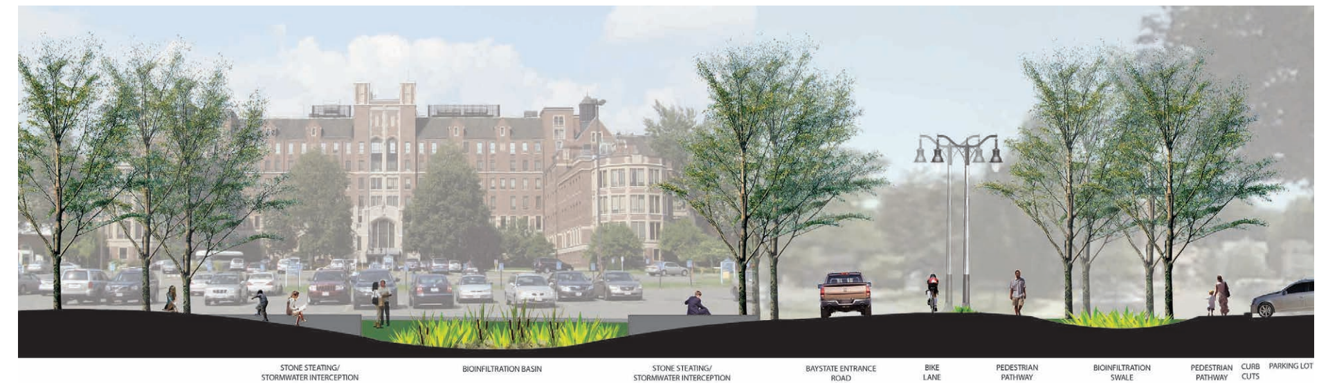
Installing an infiltration landscape by Baystate's main entrance can help mitigate stormwater runoff from neighboring parking lots. Stormwater runoff, which currently contributes to Combined Sewer Overflows, is an expensive issue Springfield is trying to remediate. In addition, this landscape can act as a comfortable outdoor seating area for Baystate employees on lunch breaks.
