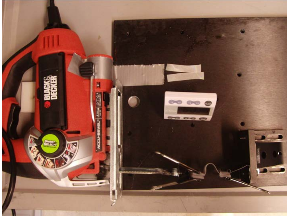
Figure 3.9: Photograph of cyclic testing apparatus. Custom made cyclic testing apparatus with a Black&Decker® jig-saw. The composite was cycled to a bending radius of 3.1 mm through a rapid deformation (10Hz) over 10,000 testing cycles
