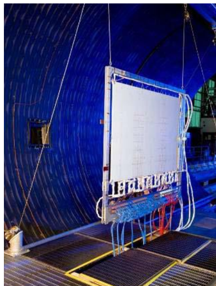
Figure 1.31: Second generation Radiator Demonstration Unit (approx. 3 ft by 5 ft) in GRC Vacuum Facility #6 [45]
