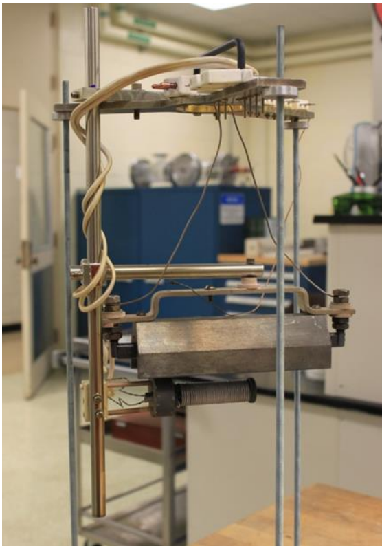
Figure 3.17: Heater assembly used for brazing (left): heater coil that supports and heats the sample, and an IR lamp above for added heat. With mounted sample (right).
