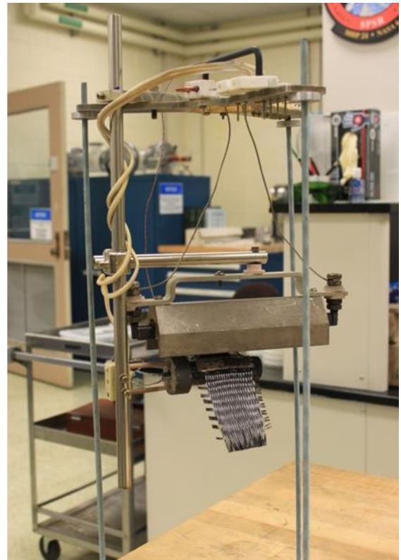
Figure 3.17: Heater assembly used for brazing (left): heater coil that supports and heats the sample, and an IR lamp above for added heat. With mounted sample (right).
