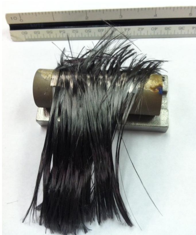
Figure 3.7: Test article A with an unwoven carbon fiber fin
