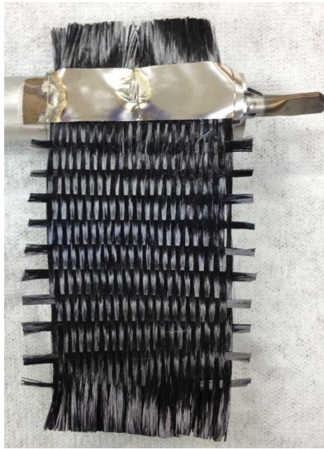
Figure 3.21: Test article E consisting of a heat pipe with a hand-woven fin
