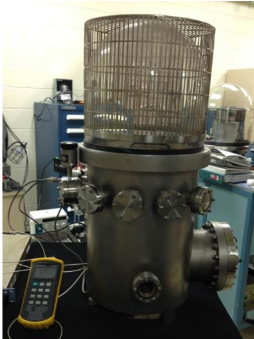
Figure 3.16: Bell jar vacuum chamber at MSFC used for brazing and testing
