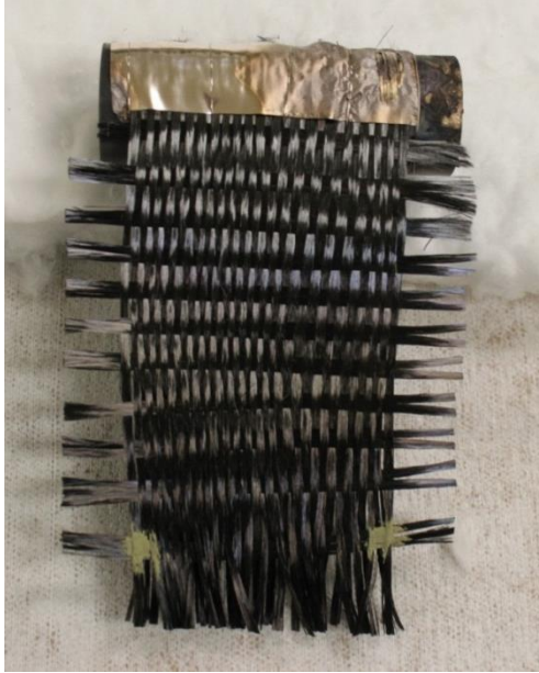
Figure 3.9: Test article C with a fiber fin generated using the second weaving method
