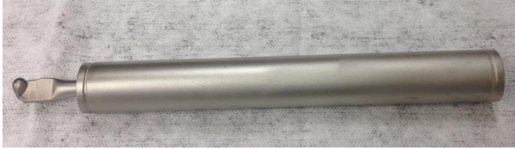
Figure 3.36: Six-inch long sodium heat pipe fabricated at NASA GRC
