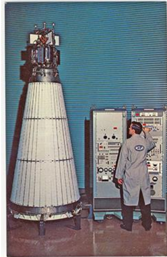
Figure 1.5: NASA's SNAP-10A spacecraft with a nuclear reactor at the top [16].
