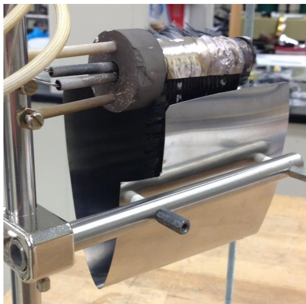
Figure 3.20: Stainless steel reflector added to the heating assembly for brazing
