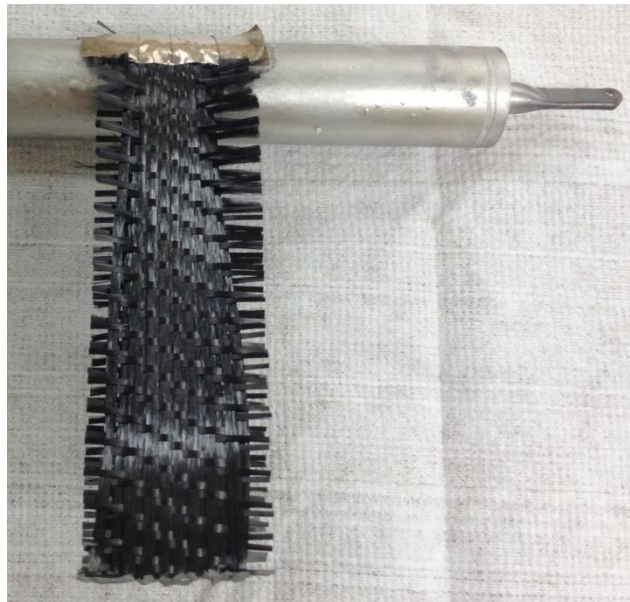
Figure 3.21: Test article E consisting of a heat pipe with a hand-woven fin
