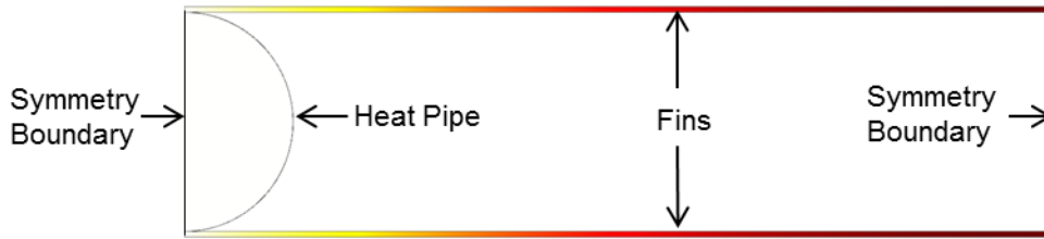
Figure 5.2: Heat pipe with the two parallel fin configuration used in thermal models accounting for radiation heat transfer between surfaces and the symmetry boundary on the right
