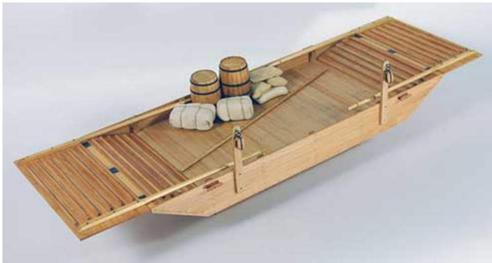
Fig. 10. From: John H. Earl, "Colonial American Ferry," [ http://www.modelboatyard.com/ferry2.html ,] February 9, 2008. While this model is more elaborate than the simple scows discussed in this paper, it provides a good visual for understanding the basic shape of these boats.
