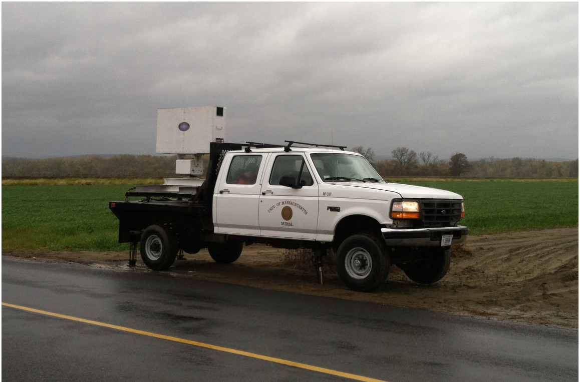
Figure I.1: The Phase-Tilt Weather Radar during an observing run in Hadley, MA on 31 October 2013.
