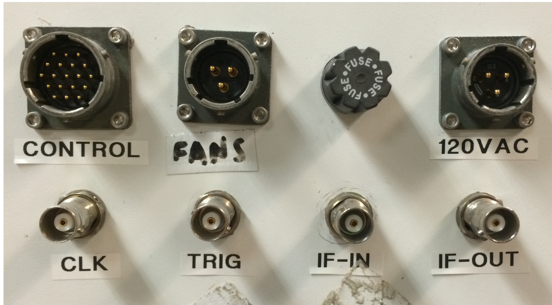
Figure 1.4: Connections on the side of the radar enclosure. Top are military connectors for power, as explained in Section 1.4.1, while the bottom are BNC connectors for transmit, receive, trigger, and clock, connecting to the Pentek transceiver.
