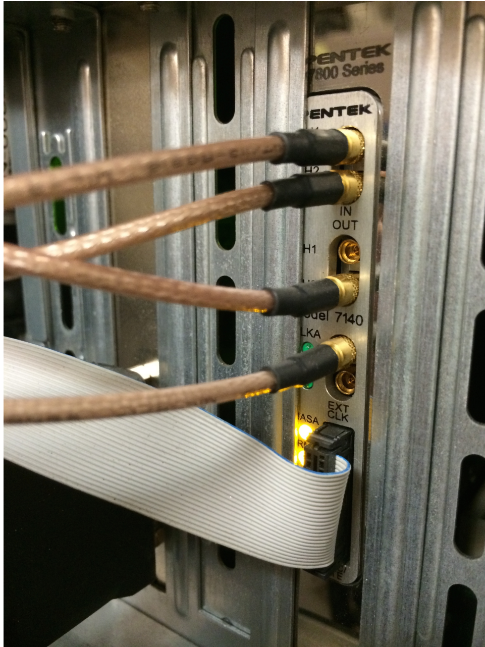
Figure 1.5: Picture of the Pentek PCI card in the back of the host computer. The top two connectors are for transmit (the bottom of the two is not used). The third connector down is receive, while the bottom is the input for a clock. Only one line on the ribbon cable is used, which is the trigger input from the FPGA.
