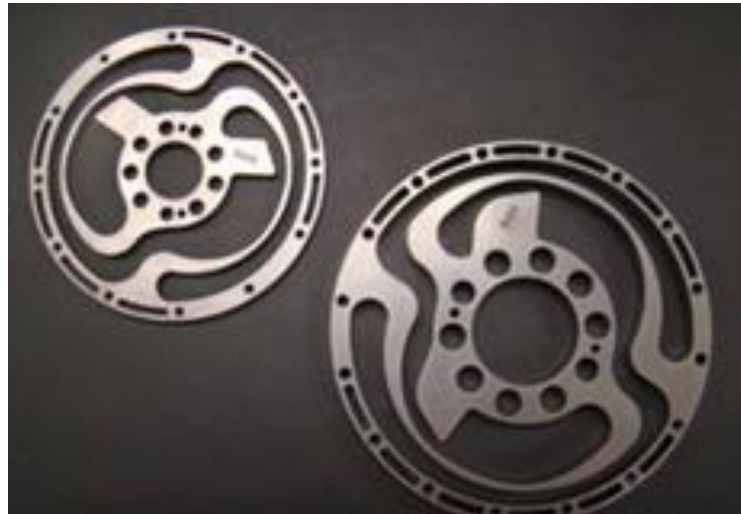
Figure 2.9 Springs used in Robonaut 2's SEAs [15]
